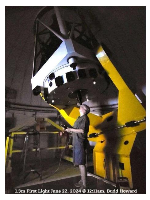
First Light of the new 1.3m telescope occurred on Saturday June 22, 2024 at 12:11am, just after midnight. The initial out of focus images exhibited nice concentric "donuts" with the secondary obscuration perfectly centered. After focusing on the bright star Vega a beautiful burst of radiant light appeared with no image distortions. To DFM Engineering's credit their mechanical alignment of the optics were pinpoint accurate requiring no additional mechanical/optical adjustments!
